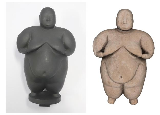
Figure 4: (Left) Photos of the replica of the Female Figurine obtained with FDM 3D printing technologies and spraypainted with a Graphene conductive coating. (Right) Visualization of the Female Figurine inside the virtual environment with its original appearance.
