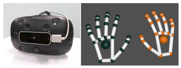
Figure 2: (Left) Leap Motion device mounted in front of the headset of the HTC Vive. (Right) Stylized model of the hands tracked by the Leap Motion.
