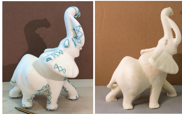
Figure 12: (a) The mold is tied together before the resin is poured; (b) the result of the cast of the elephant model.
