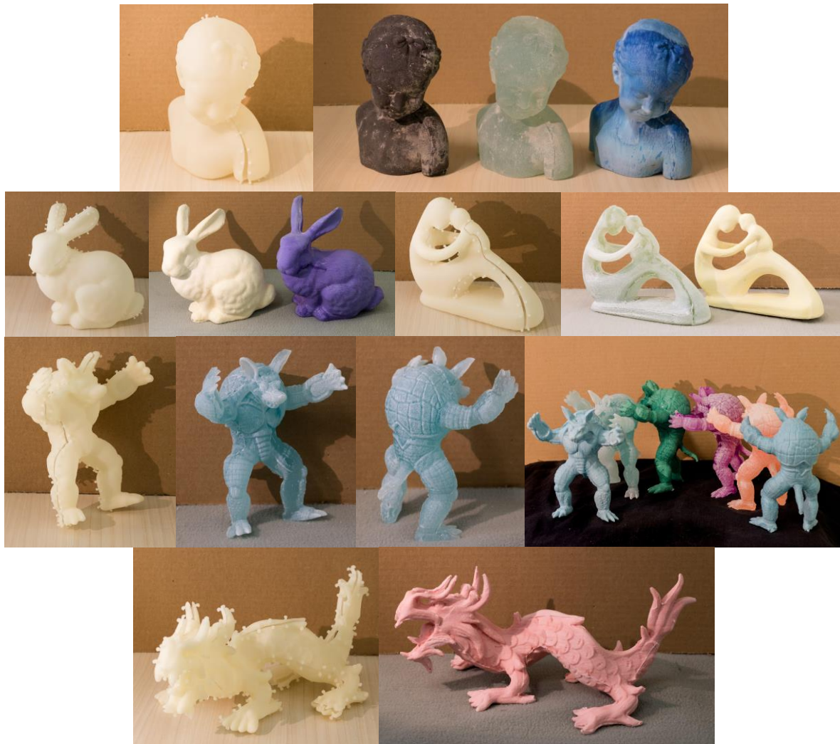
Figure 16: Molds and casts obtained for the bimba, the bunny, the fertility, the armadillo and the dragon models.
